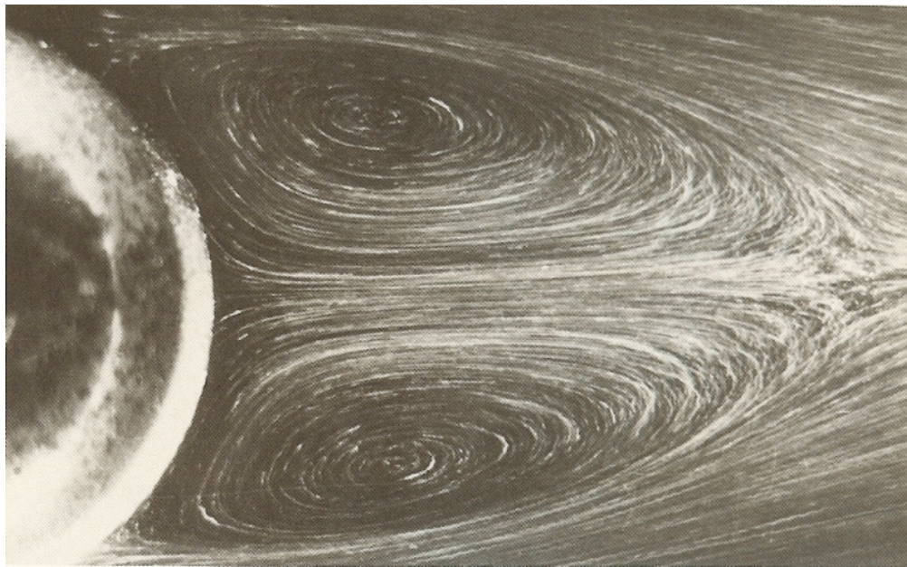
Figure 3: Low speed flow of water past a sphere at Reynolds number R = 118 . Water circulates back to the low pressure region at the rear of the sphere after it separates. Photo 53, page 33, Album of Fluid Motion.
